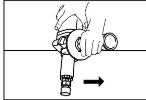
Turn the tool on without the wheel point making any contact with the workpiece and wait until the wheel point attains full speed. Then apply the wheel point to the workpiece gently. To obtain a good finish, move the tool in the leftward direction slowly.
