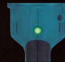
Solid Green indicates that current can be applied to the circuit. (GA9050R / GA7050R)
