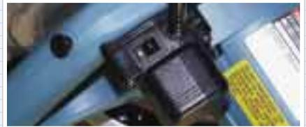
On-Off switch for exclusive use of lamp works independently; independent of the On-Off switch for the motor.
