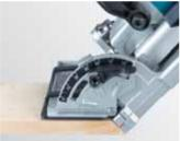
Angle adjustable fence can be locked in any position between  $0^{\circ}$  and  $90^{\circ}$  with positive stops at  $0^{\circ}$ , 45° and 90°.
