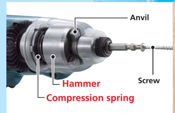
First, the counter torque from screw reduces the rotational speed of Anvil.
