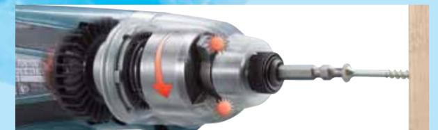
Finally, Hammer delivers enormous impact power onto Anvil, and the tool drives a screw with the high torque which rotational power alone cannot produce.
